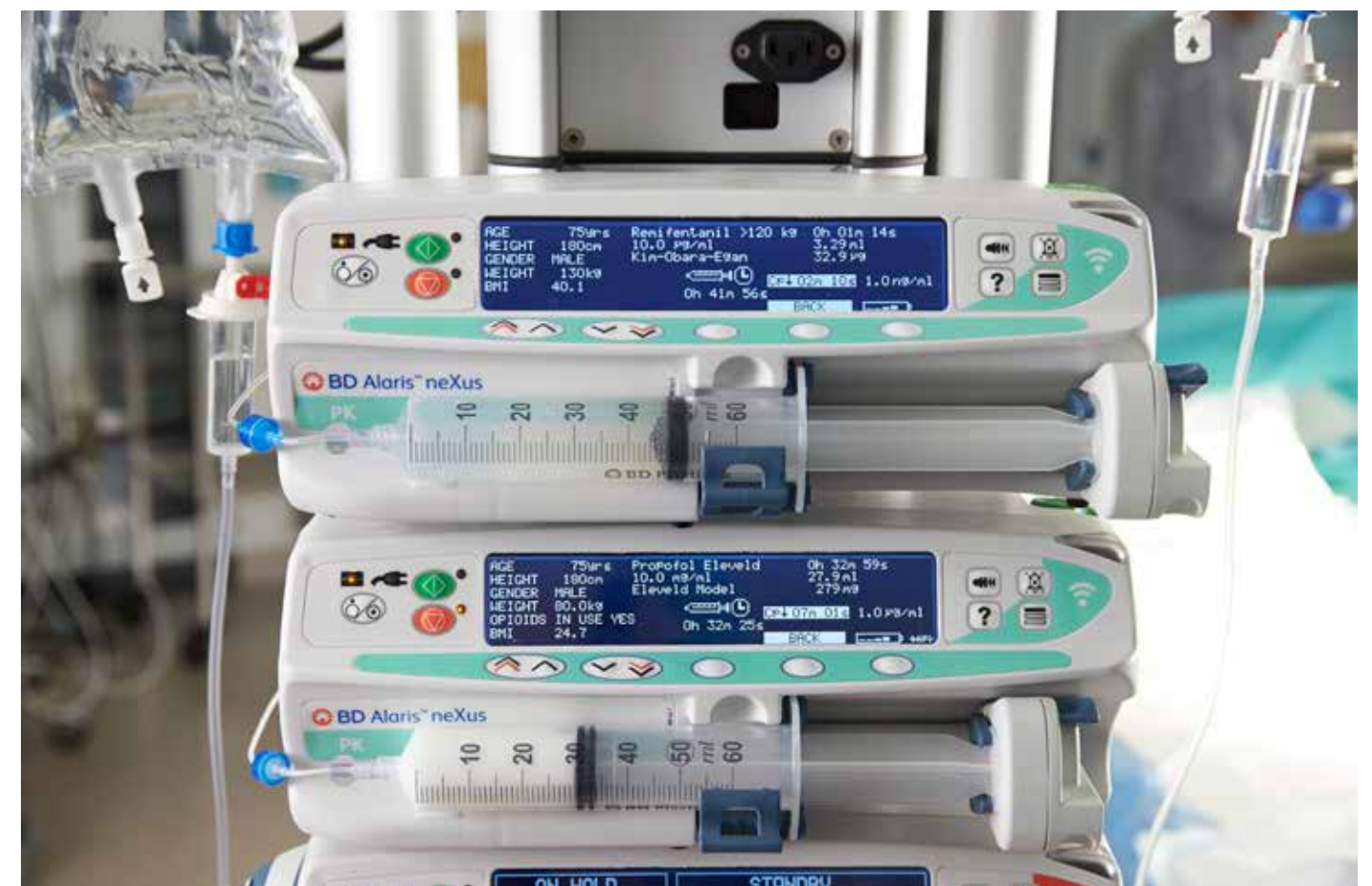
TIVA and TCI requires two pumps- one for the hypnotic infusion and one for analgesia
